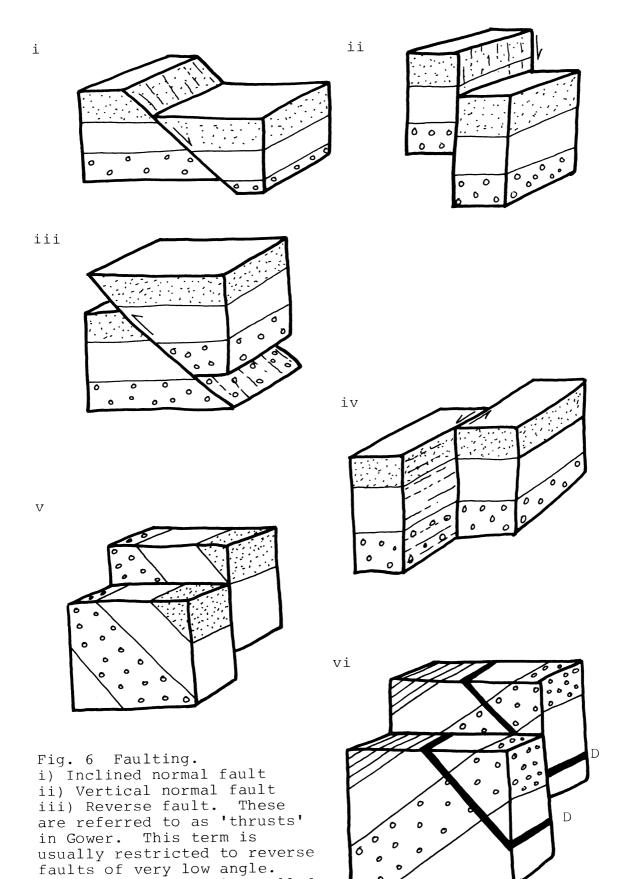
'tear' fault). v) The effect of normal vertical fault on inclined strata. Note apparent lateral displacement along fault, though movement vertical. vi) scenario as for (v), but presence of dyke D shows fault-movement was vertical, since its apparent lateral shift is in opposite direction. True lateral shift as in (iv) would have affected it in the same way as the beds.
